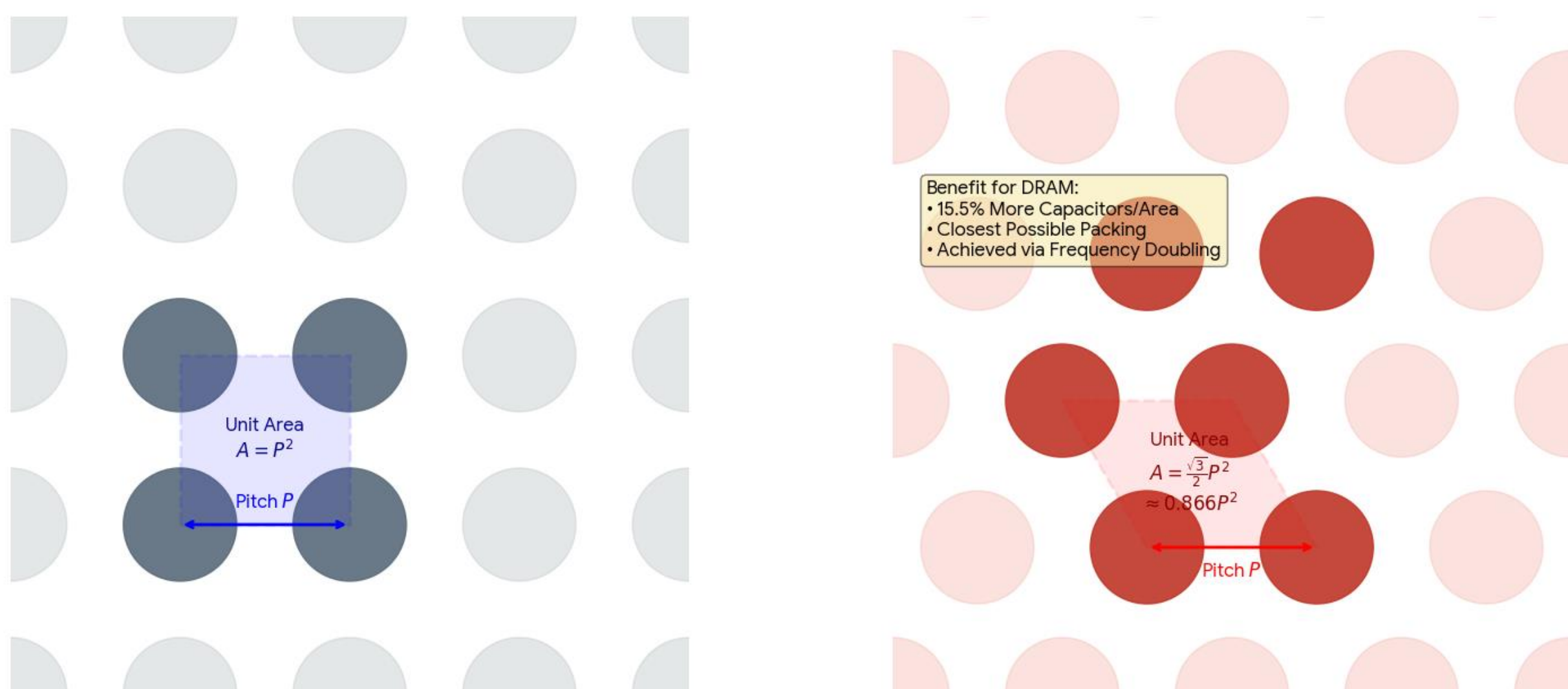
Figure 1. Triangular lattices allow for denser packing. Left: Conventional square lattice arrangement; Right: triangular lattice arrangement.
